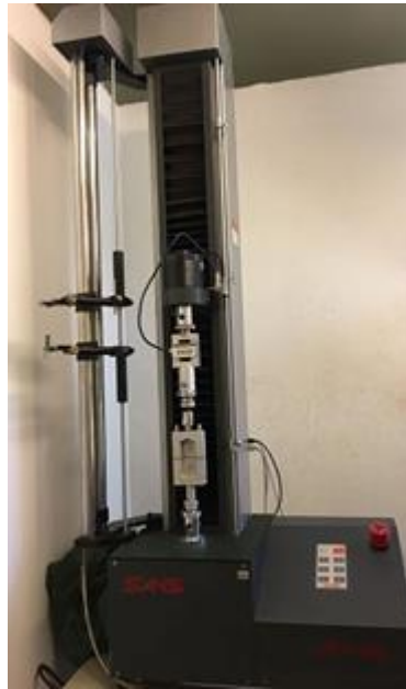
Fig. 2: Universal testing machine (MTS SANS CMT 2000 5KN)
